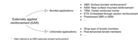
Figure 17.1-1: Externally applied reinforcement
